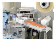
4.Wrapped sushi comes out automatically.
