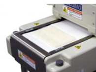
1.The machine spreads sushi rice onto the forming sheet
