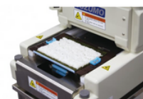
2.The machine spreads a sheet of sushi rice on the Nori
