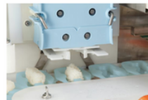
1.Initial stirring to separate grains of rice and forming of rice balls
